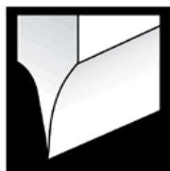
Conventional Hollow-Ground Edge
